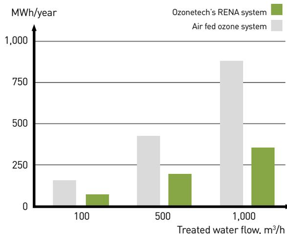
The RENA system range ensures sustained overall efficiency of minimum 25 grams dissolved ozone/kWh.
